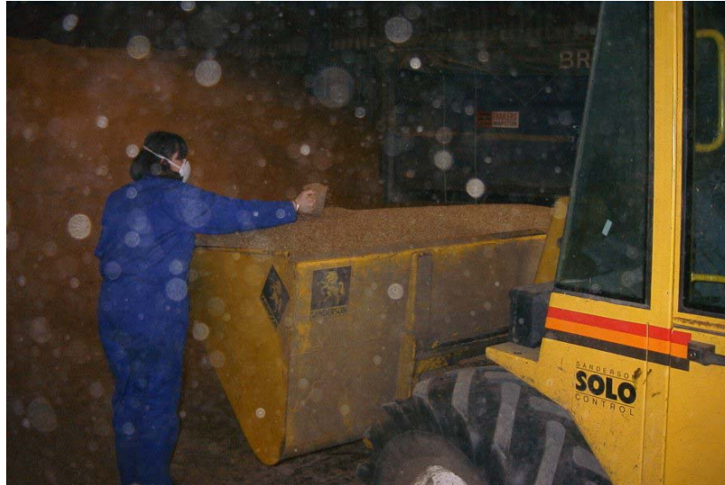
Figure 2. Collection of a sample from a front loader bucket.
