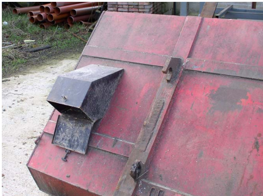
Figure 4. Automatic sampler with collecting box open.
