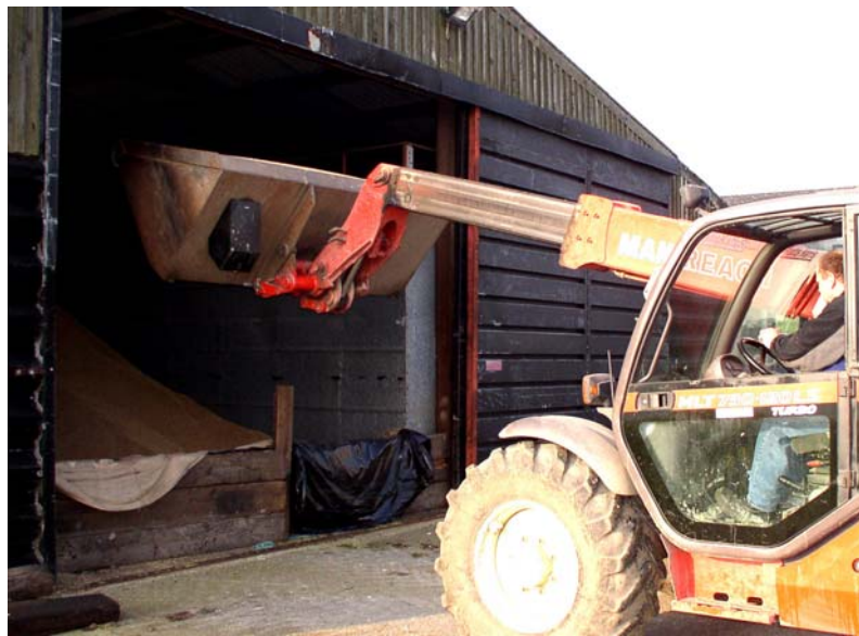
Figure 3. Automatic sampler fitted to a front loader bucket
